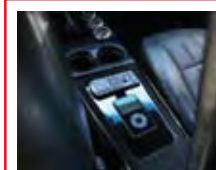
The iPod is flush-mounted into the console and hidden when the lid is closed.
